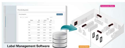
Concept display of the connection between the label management software, communication station, and terminal display in a mock-up retail environment
